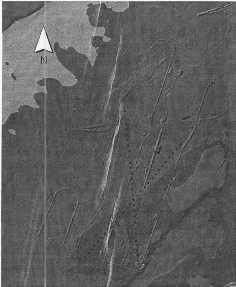
Figure 2. Synthesized topography of a firing range at Fort Drum Military Reservation, New York (2-m grid resolution). Dots indicate the snow depth survey locations taken on 4 January 2001.
