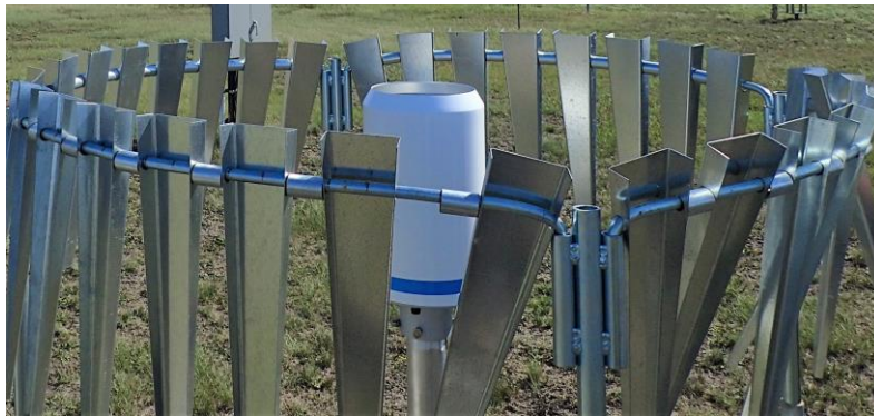
Figure 1. Single Alter shielded Lambrecht rain[e]H3 heated tipping bucket / weighing gauge installed at the Bratt's Lake (SK) supersite.
