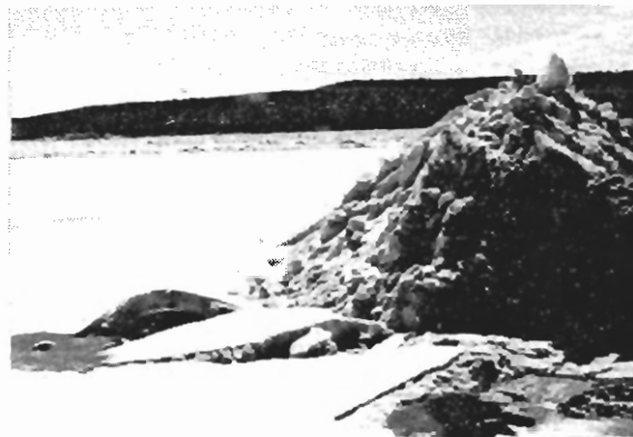
Fig. 3 Grounded ice sheet showing evidence of creep buckling and crushing.
