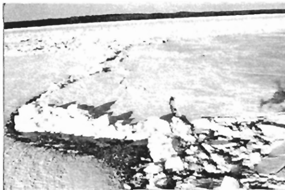
Fig. 9 A large ice floe (right) overrides the intact ice (left) showing evidence of vertical bending failure.
