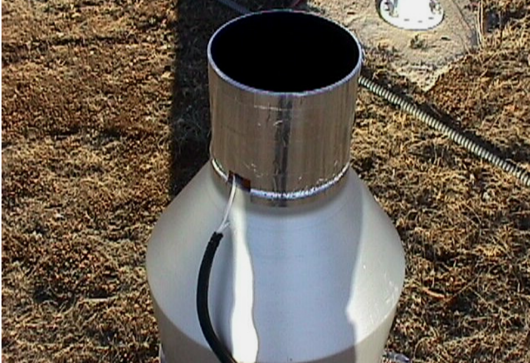
Figure 4. A T-200B Geonor gauge showing the upper Kapton flexible heating element. A similar heating element is affixed to the section of the orifice below the shoulder of the gauge.
