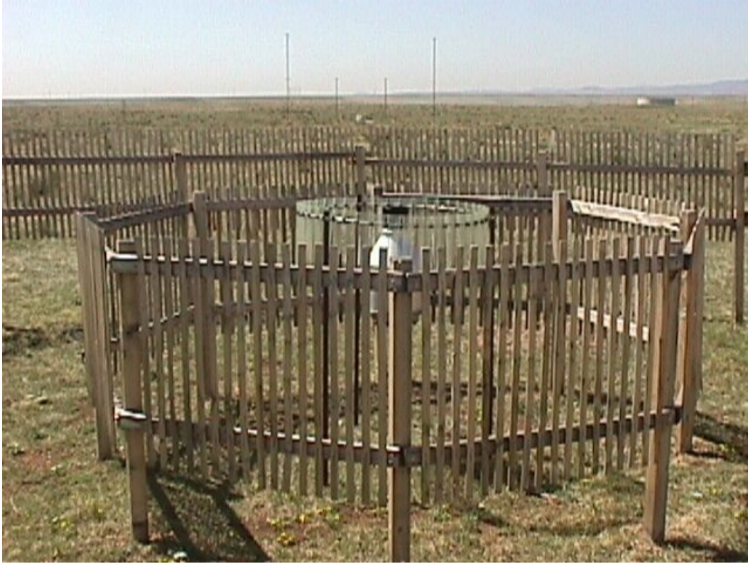
Figure 2. A view of the DFIR from just inside the outer shield. In the foreground is the inner shield and, in addition, an Alter shield surrounds the gauge.
