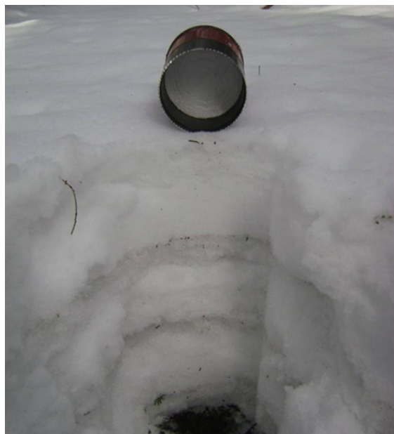
Figure 6. Snow density profiles were taken with a 65 mm diameter by 60 mm deep anodized aluminum cylinder with serrated surface to help cut through ice layers. Each 100 cm 2 sample was placed in a Ziploc bag and massed to the nearest 0.1 grams. Densities ranged from 150 kg m -3 for newly fallen snow at the top of the pits to 800 kg m -3 at the base of pits at the end of the season.
