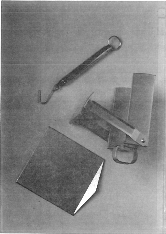
Fig. 1 The Swedish snow sampler
