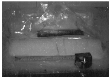
Figure 2. Ice core segment from 1150 masl. Note the ice layers in the firm.
