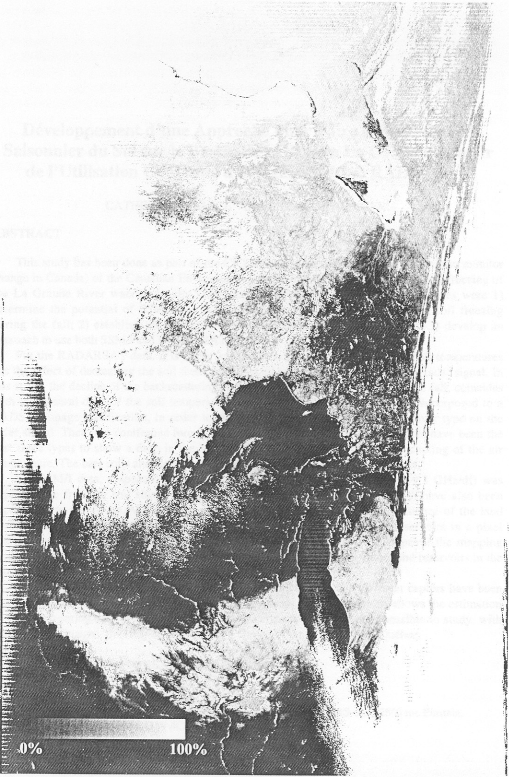
Figure 11. Fractional snow cover for the 08 April 2000 MODIS swath covering northern central North America. Clouds are shown in white.
