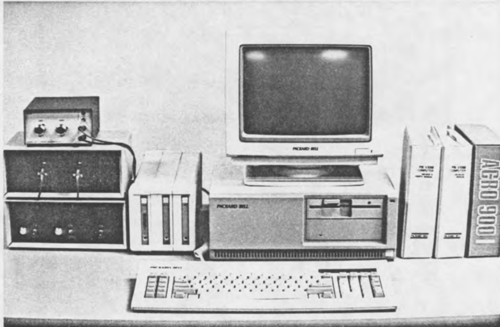
Photograph 4. The automation equipment used by Frank H. Theakston & Associates Inc.. On the left power supplies and switching relays for the scanivalves (not shown). Next the data logger and then an 8088 8 MHz MS-DOS microcomputer used to control and record the experiment.
