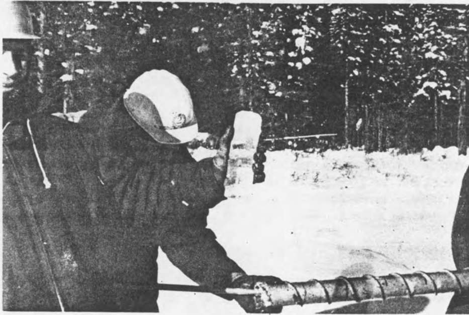
Fig. 7 - Ice core having 2 inches white ice and 5 inches clear ice. Clearing tool being used to remove ice cuttings from inside of tube.
