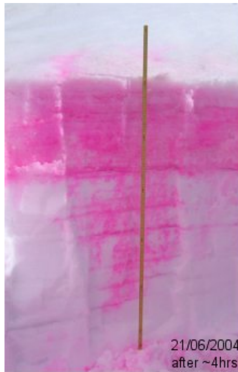
Figure 3: Ice layers causing retention of percolating meltwater and lateral variability of flow.
