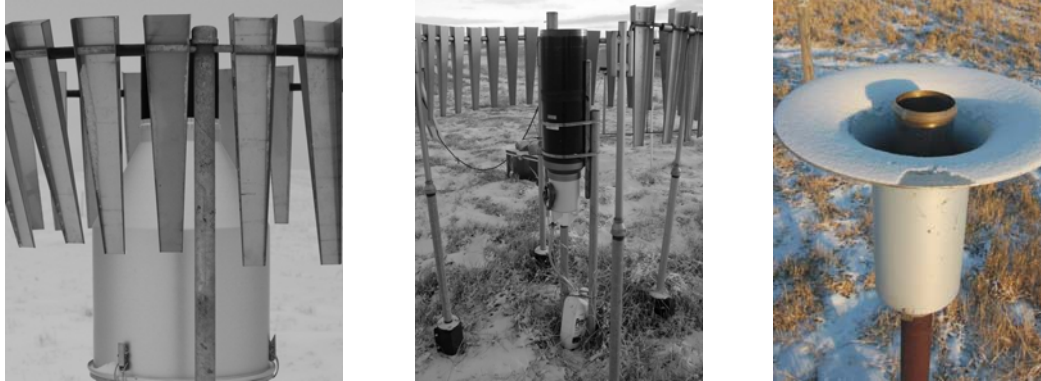
Figure 1. Geonor T200-B with Alter-shield (left) Campbell Scientific with Alter-shield (centre), and Nipher-shielded MSC manual gauge (right).
