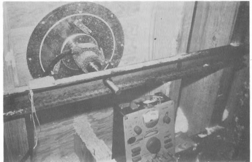
Figure 5. Lateral pressure cell installed on the wall of the truss enclosure.
