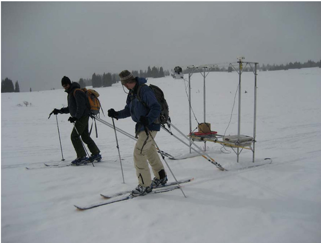
Figure 1. Aluminum radar sled, with FMCW radar (4-18 GHz) mounted on far side at a height of 2.3 m and an incidence angle of 30 degrees. Radar is also mounted in center of sled at 0 deg. to measure snow between skiers. Sled is attached to skiers with a rigid harness system, and also contains a survey-grade GPS system.
