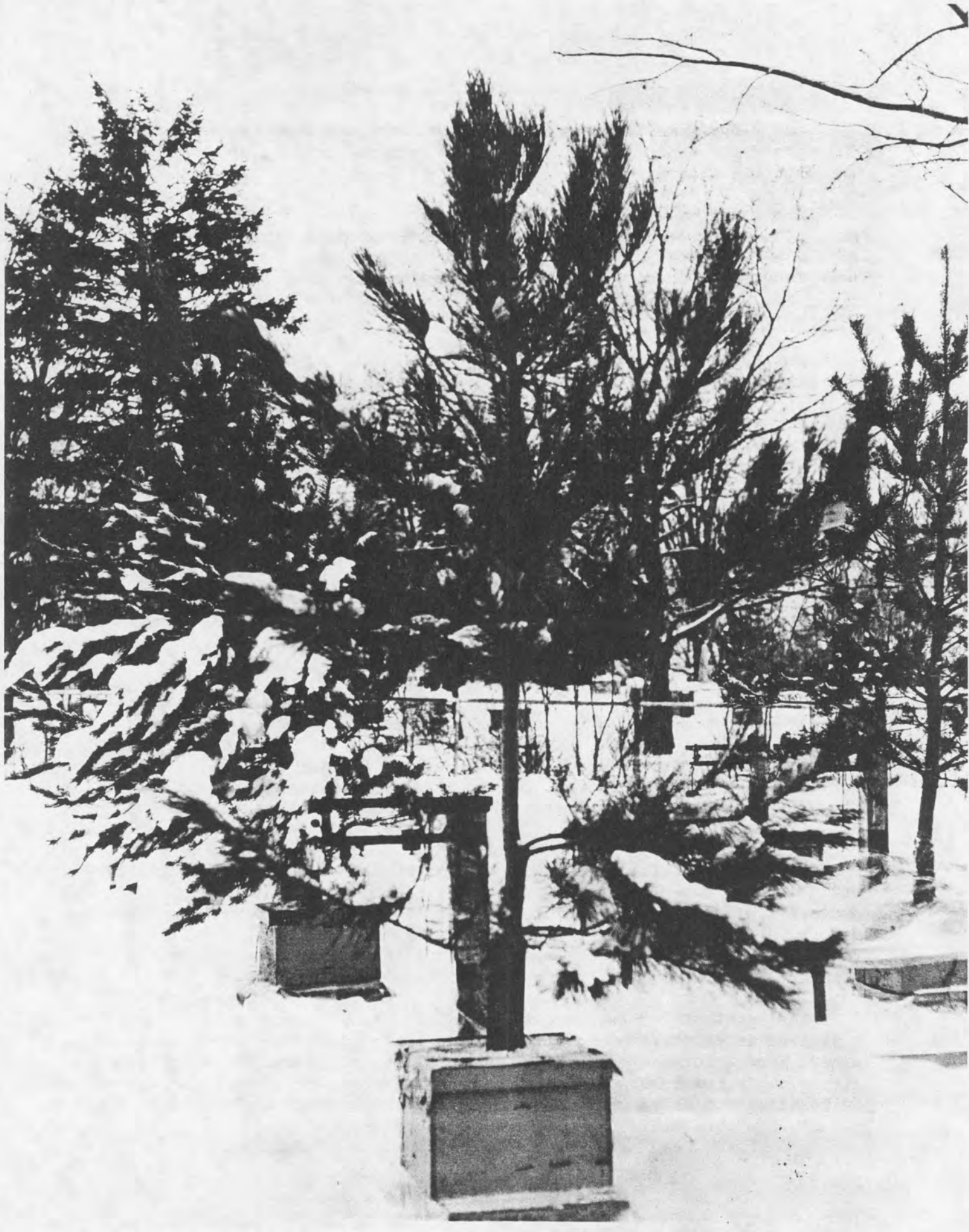
Figure 1.--Experimental installation for snow interception.
