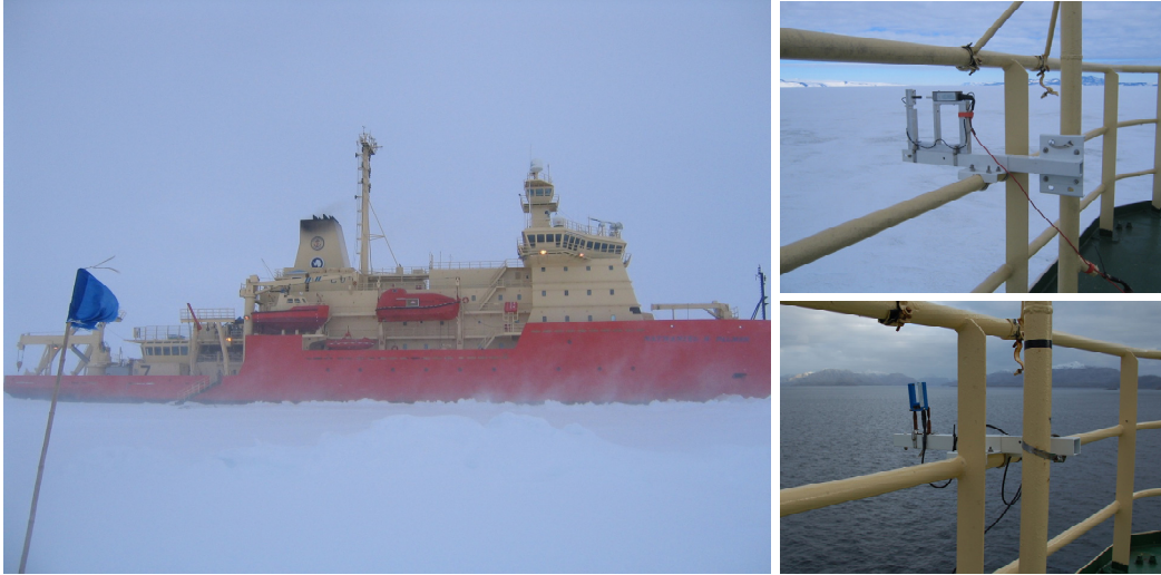
Figure 2. (left) R/V Nathaniel B. Palmer . The observation tower on which the two particle counters (right) were installed is on the right in this photo, above the bridge. Photographs of the particle counters were taken from the port-side of the observation tower roof facing forward, showing the mounting arm and particle counters pointing towards the bow, in alignment with the ship's long dimension. During cruise NBP0702 the particle counter shown on the upper right was on loan from York University. The counter shown at lower right was manufactured by the Wenglor Corporation, and was used during cruise NBP0709.
