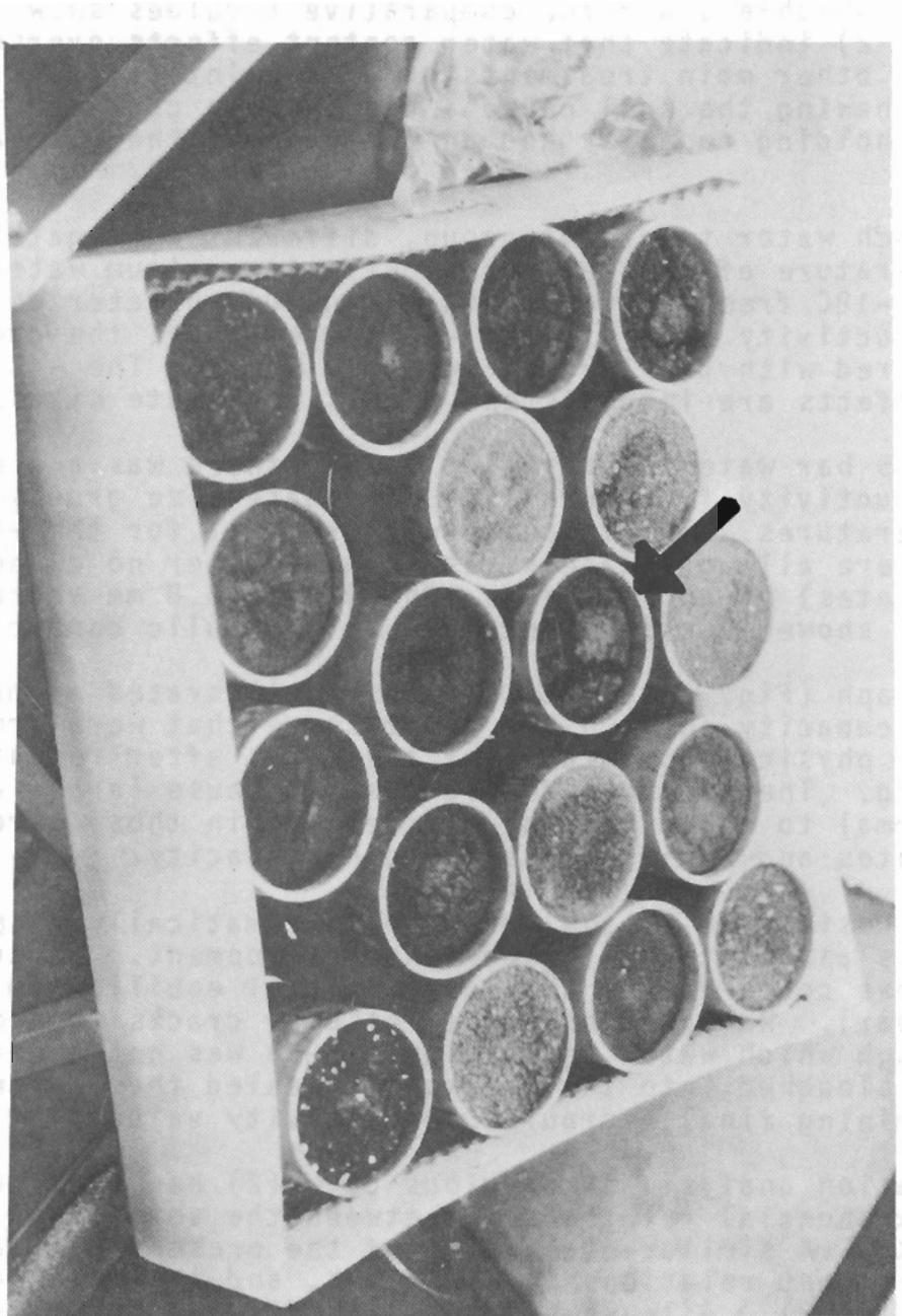
Figure 1. Soil cores with initial water equilibrium values of maximum water-holding capacity and 0.5 bar of pressure just after the -18°C freeze-thaw treatment.
