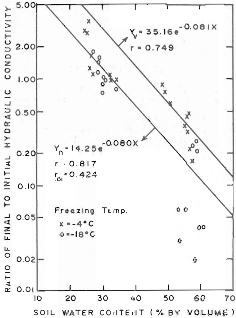
Figure 2 Semilog plot of the relative change in soil hydraulic conductivity normal to the direction of freezing after freezing and thawing soil cores at different soil water contents.
