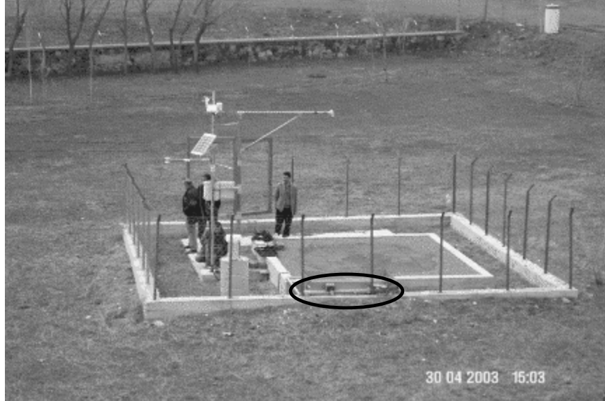
Figure 3: General overview of Guzelyayla Automatic Snow Pillow and Automatic Weather Station (Circle indicates the location of the snowmelt lysimeter).
