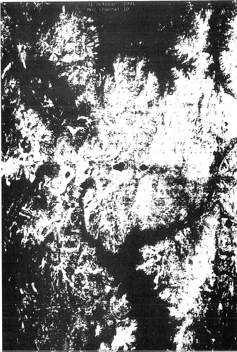
3. Snow-covered area as determined from MAS channel 10 (center wavelength 8.8 \mu\text{m} ) data obtained on 31 October 1991 in the Sierra Nevada Mountains, California. According to this classification, the snow-covered area comprises 42 percent of the entire scene.
