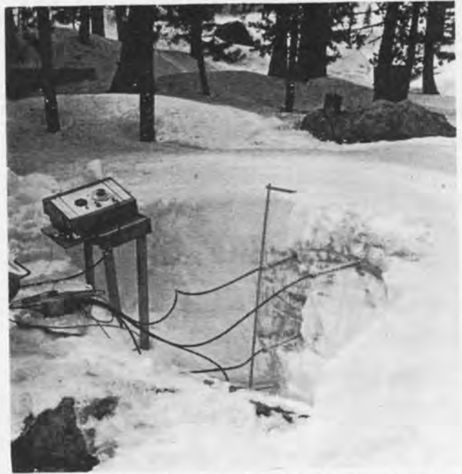
FIGURE 3—The Snow Moisture Meter with probes inserted in a snow profile at flow zone points previously identified with fuchsine dye.
