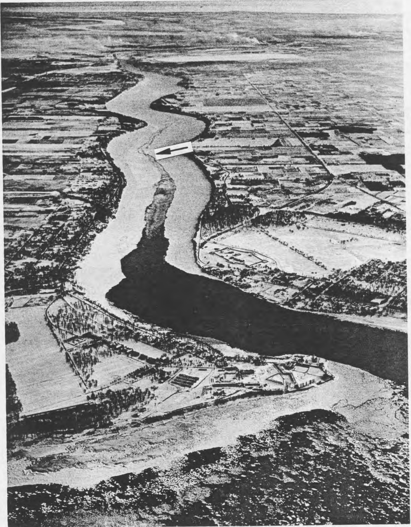
LOWER RIVER ICE JAM LOOKING UPSTREAM ICE COVER BEING REMOVED BY ICEBREAKER (SEE ARROW) 14/I/64
