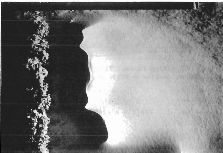
Fig. 18. Run 10-25-1, short simulated row of trees (scale is 0.3 m long), flow left to right.
