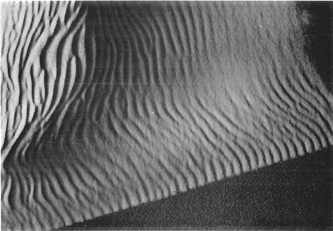
Fig. 8. Close-up view of cornice formation and edge of drift, Run 5-1-1, flow left to right. The ripple pattern, of course, is not to scale. Ripple wave length is sufficiently short so that gross drift features are not affected except, perhaps, near the cornice.
