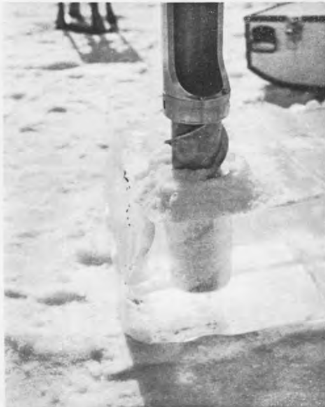
FIGURE 3 — Ice cuttings move upward along helix barrel as coring auger penetrates ice block.
