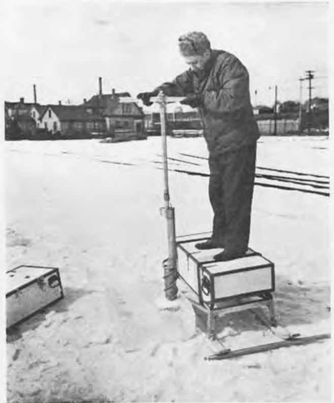
FIGURE 1 — Coring a block of ice. T-handle is being used to rotate auger in place of the brace normally used. Additional drilling equipment components shown are extension rod, core remover barrel, and helix barrel.
