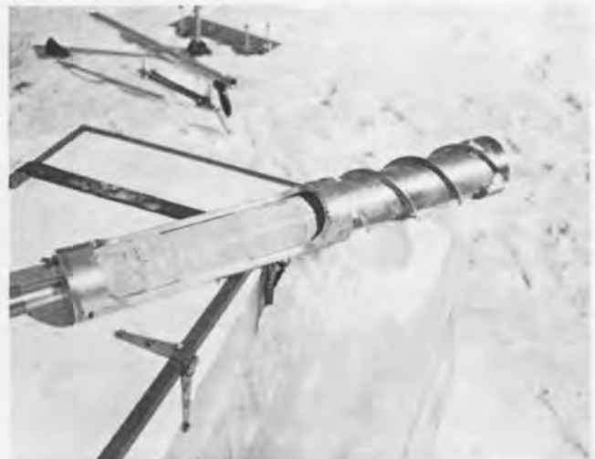
FIGURE 2 — Ice cores may be removed by sliding them up into the core remover barrel as shown.
