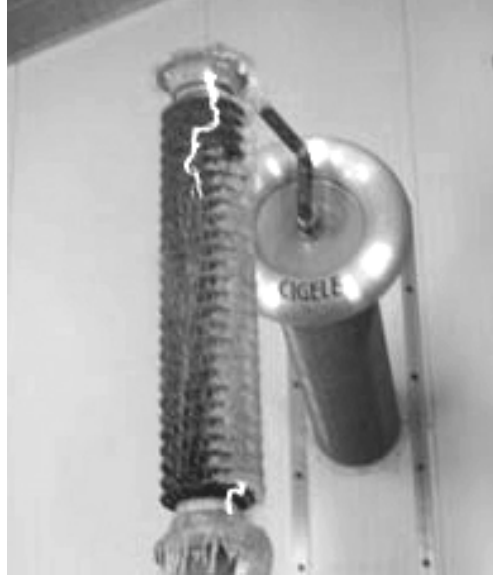
Figure 7. Two arcs are established at both ends of the ice-covered insulator
