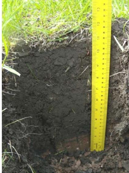
Figure 4. Soil Profile at Site 1. The upper 25 cm are loam/soil with an under layer of clay (about 5 cm of clay are showing in the photograph). The soil pit was dug in the summer months.
