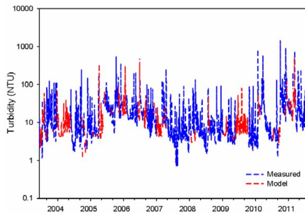
Figure 2. Continuous time series (2003–2011) of average daily turbidity at Coldbrook showing the range in observed and interpolated missing turbidity values
