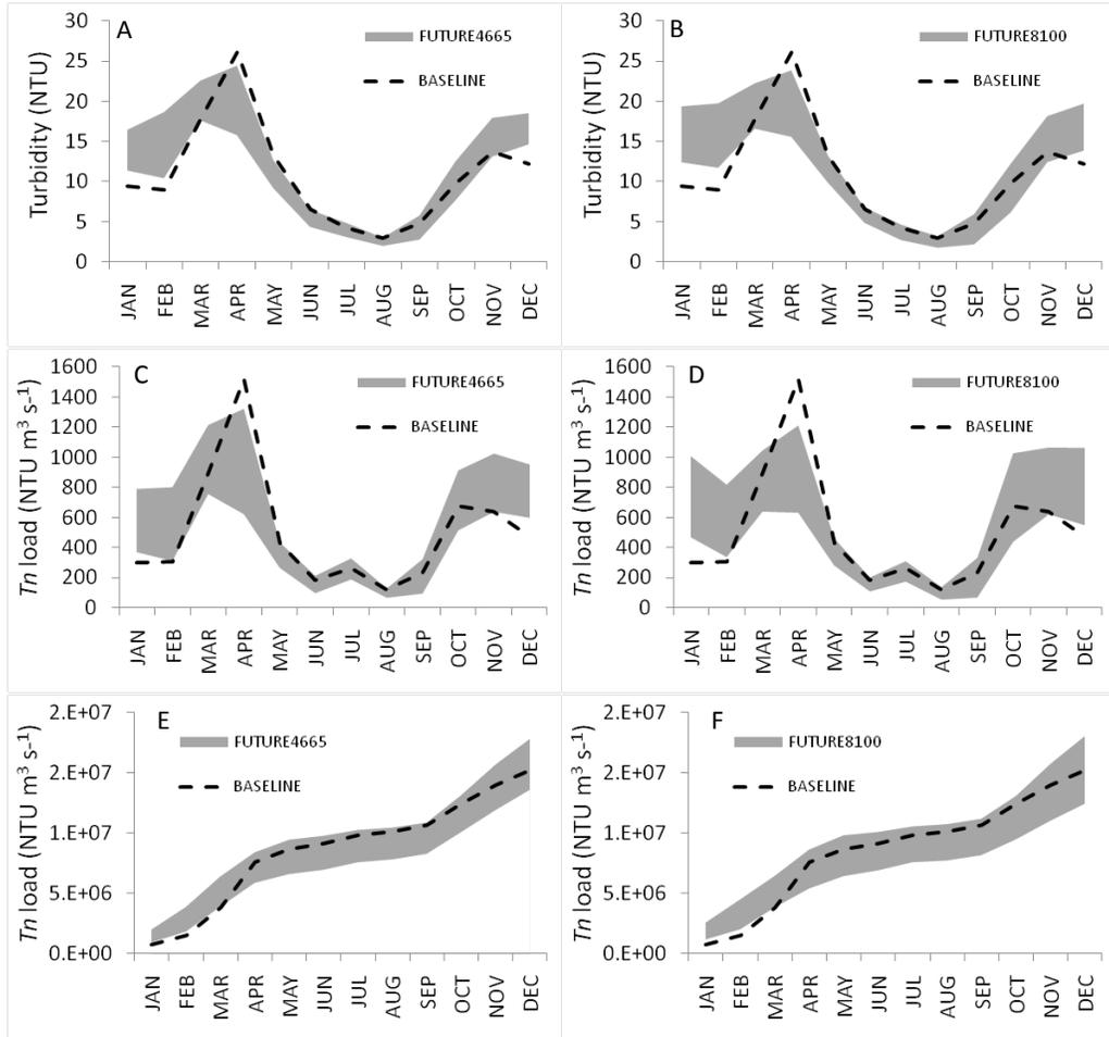
Figure 3. Comparison of baseline vs. future ambient stream turbidity for the 2046–2065 period (A) and 2081–2100 period (B); projected change in average ambient turbidity load by month for the 2046–2065 period (C) and 2081–2100 period (D); projected change in average annual cumulative turbidity loads (E and F).
