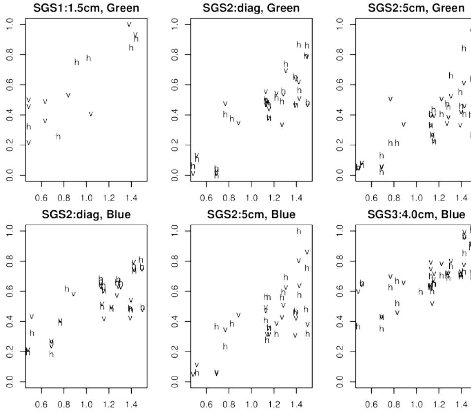
Figure 5. Normalized transmissivity,  $T_n$  vs.  $D_{obs}^*$  vs. by separation for top row: SGS-1 (green), SGS-2  $B_{HG \rightarrow VO}$ , SGS-2  $B_{VG \rightarrow V^*}$ ; bottom row: SGS-2  $B_{HB \rightarrow VI}$ , SGS-2  $B_{VB \rightarrow VI}$ , SGS-3 (blue). h: horizontal sensor orientation, v: vertical sensor orientation.
