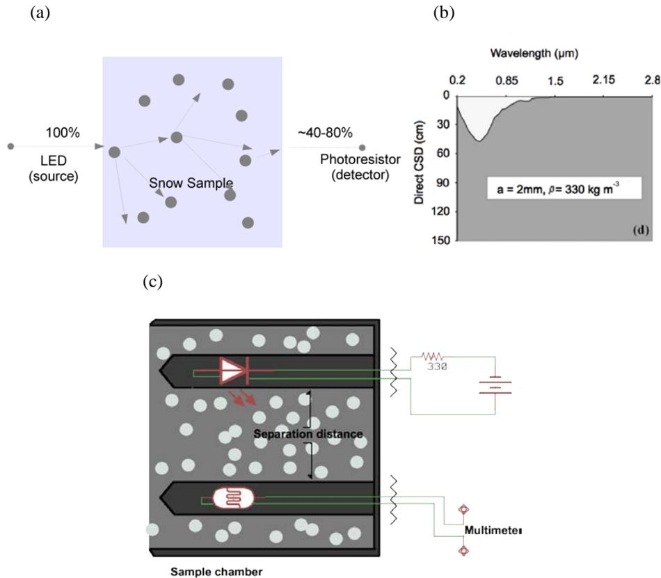
Figure 2. (a) Function of the GS probe. (b) Zhou et al. (2003a), Figure 2(d), relationship between extinction depth, wavelength, grain size, and density for natural light. (c) Schematic diagram of SGS-1 components.
