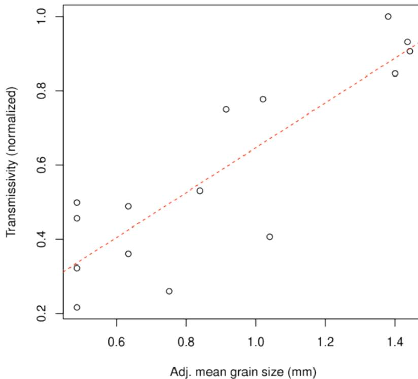
Figure 4. Calibration regression of optical loss in transmission to grain size.
