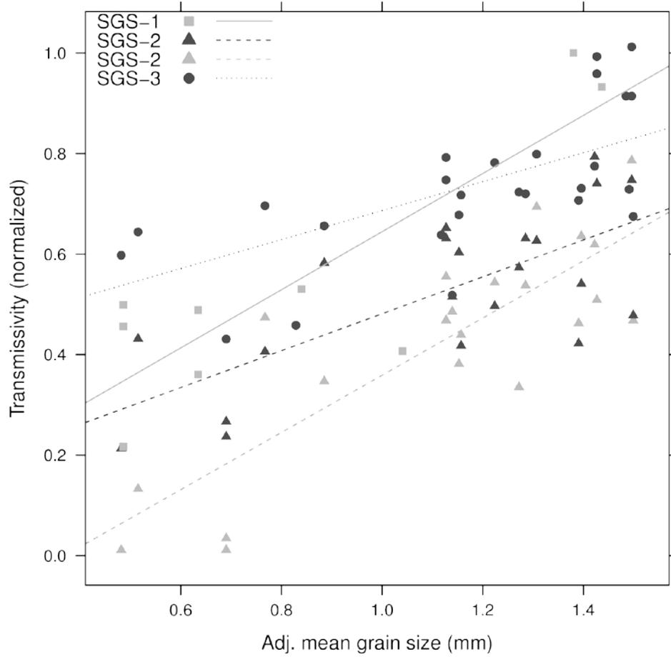
Figure 6. Grain size vs. attenuation for SGS-1, 2 (selected modes), 3. Symbol color indicates transmitting LED (light grey: green LED, dark grey: blue LED) . Lines show best fit of  $T_n \sim D_{obs}^*$  per sensor and band.
