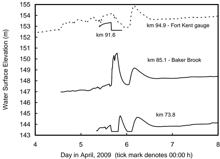
Figure 8. 2009 water level records in middle portion of study reach, Fort Kent/Clair to ~11 km above Edmundston. The loggers at 91.6 and 73.8 kms were respectively located near the small communities of Caron Brook and St-Hilaire. From Beltaos *et al.* (2011).
