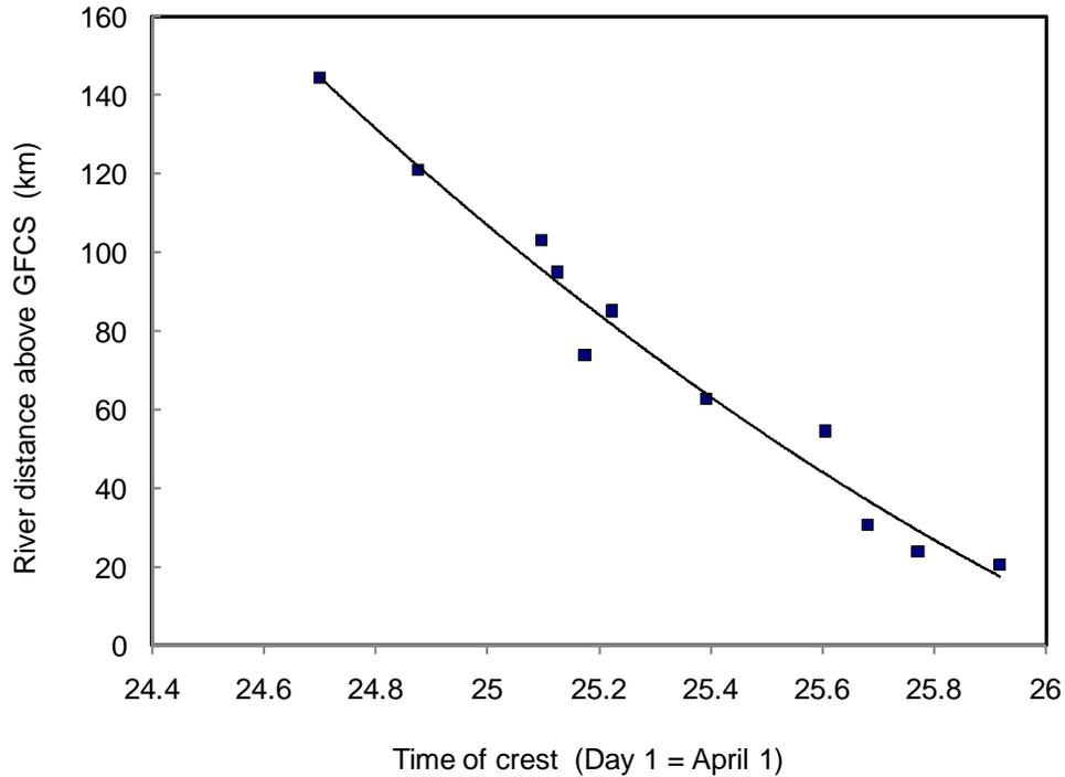
Figure 13. Plot of river distance versus the time of crest along with a polynomial fit to the data points. The slope of the line represents crest celerity in km/day.
