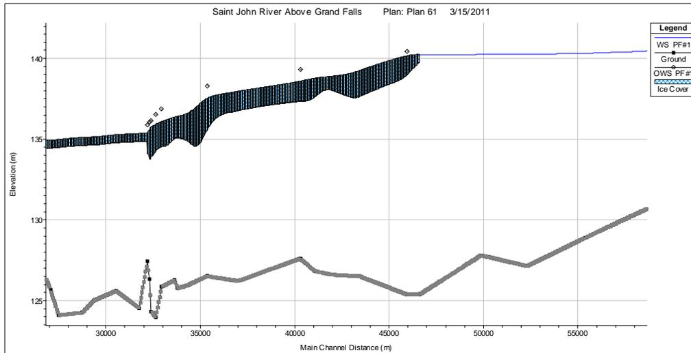
Figure 4. HEC-RAS graphical output for  $\Delta L$  of 50 m ( $\sim 1/4$  of channel width). Ice jam near Ste-Anne, 1991.
