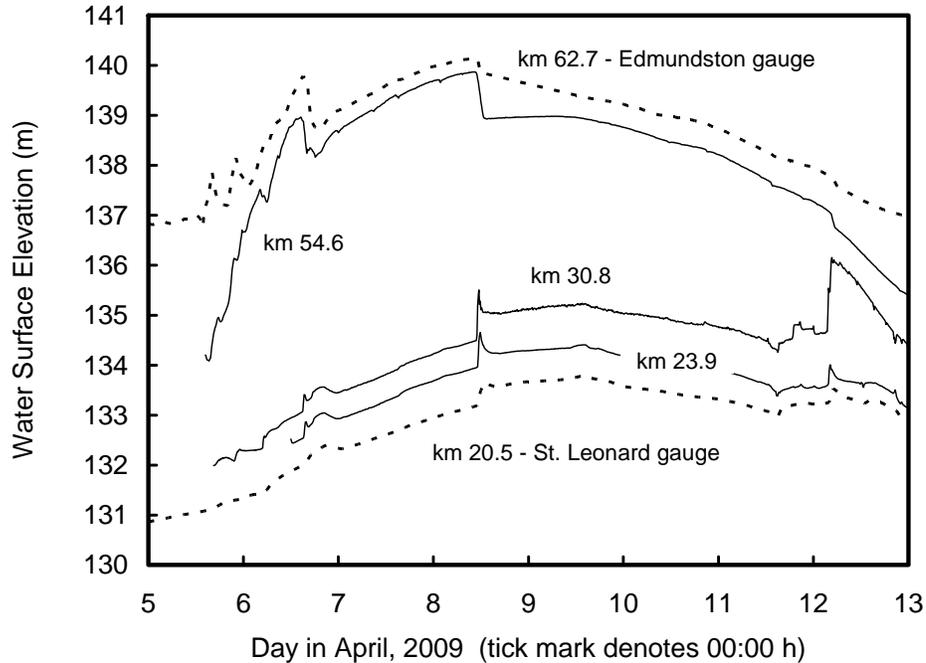
Figure 9. 2009 water level records in lower portion of study reach, Edmundston to St. Leonard. The loggers at 54.6 and 30.8 kms were respectively located near the small communities of St-Basile and Ste-Anne-de-Madawaska. The logger at km 23.9 was located slightly downstream of the mouth of Grande River. From Beltaos *et al.* (2011).
