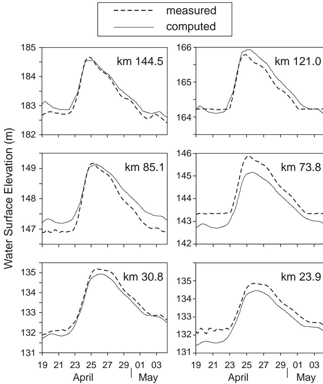
Figure 12. Examples of numerical simulations of runoff waves using the unsteady flow option of HR.
