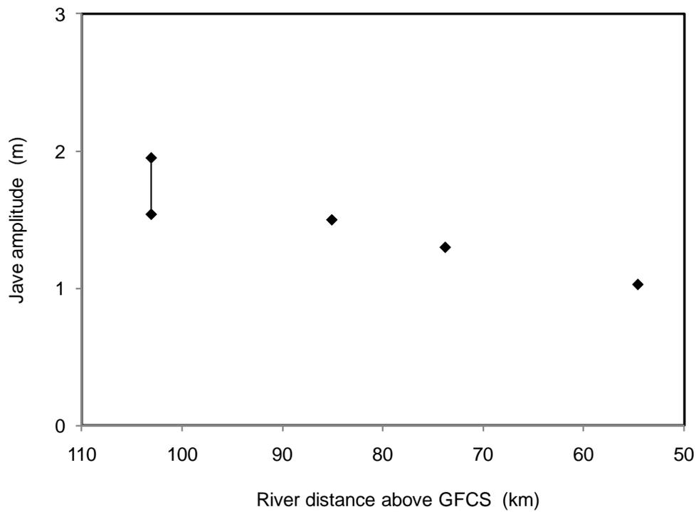
Figure 11. Attenuation of jave amplitude, April 6, 2009. The peak stage at km 103.1 may have been enhanced by downstream jamming; the jave amplitude can only be determined to within the indicated range.
