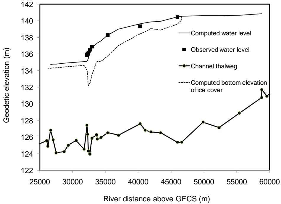
Figure 2. Model output versus measurements, ice jam near Ste-Anne, April 12, 1991.
