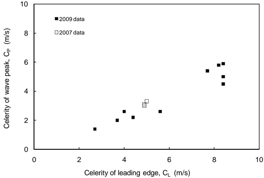
Figure 10. Celerity of jave peak ( $C_P$ ) plotted versus that of the leading edge ( $C_L$ ) for the 2009 breakup event. Note approximate relationship and ranges of respective values.
