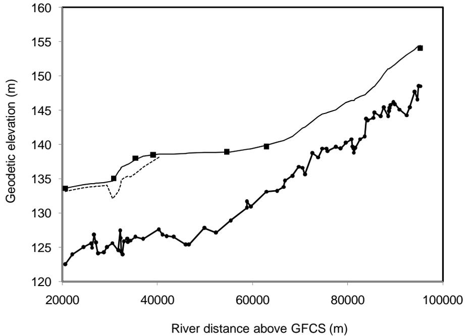
Figure 3. Model output versus measurements, April 8, 2009. Same legend as in Fig. 2. The last two data points were obtained from gauge records at Edmundston (~ 63 km) and Fort Kent (~ 95 km).
