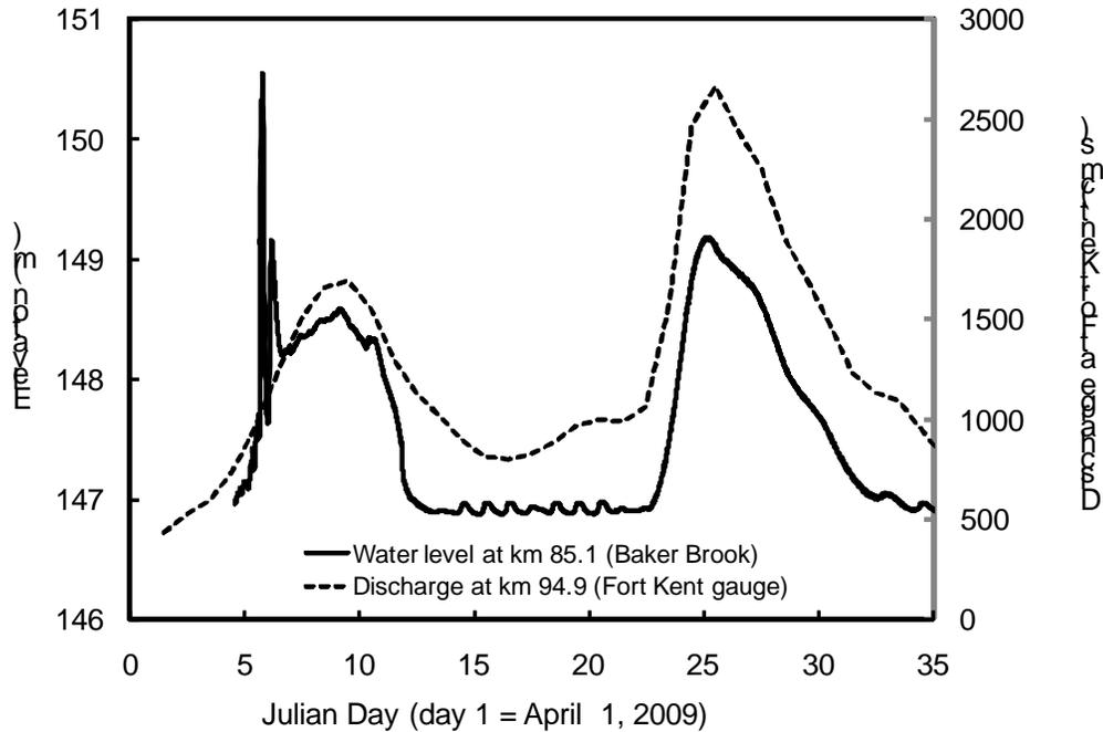
Figure 6. Water level variation near Baker Brook during April and early May 2009 as obtained from pressure logger output. Discharge is indicated on the secondary axis.
