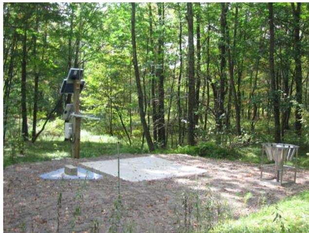
Figure 4. Introduction of SnoScale to Neversink test site along with Pluvio weighing bucket and SR50 Snow Depth Sensor, September 2009
