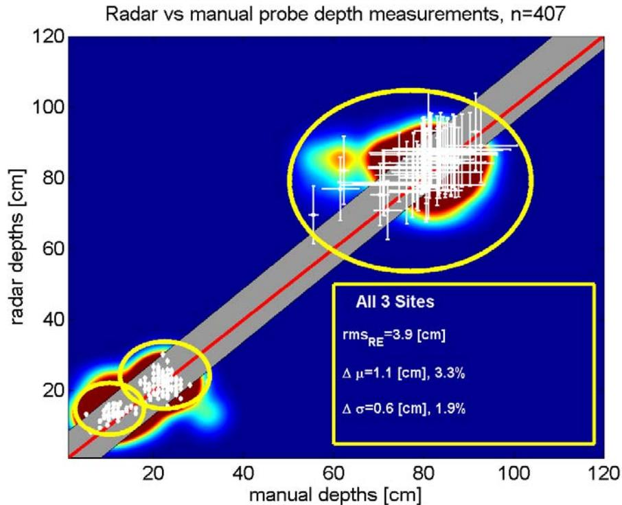
Figure 5. Comparison of manual and radar snow depths.
