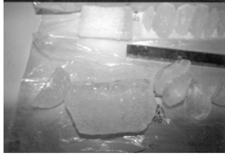
Figure 3. Ice core segment from 950 masl. Note that there is very little firn, suggesting that melt has taken place.
