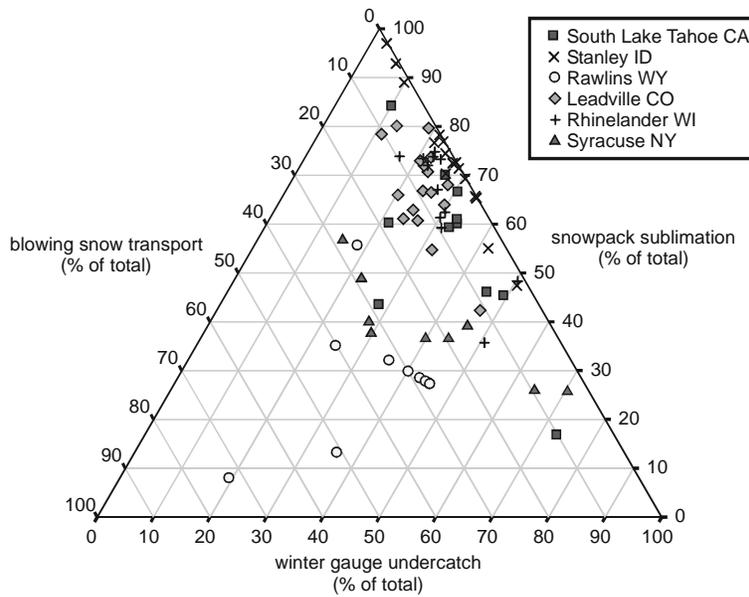
Figure 3. Distribution of monthly precipitation gauge undercatch, snowpack sublimation and blowing snow transport as a function of the sum of the three components for the three winters at the six study sites
