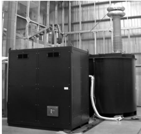
Figure 3. UQAC 350 kV alternating high-voltage system
