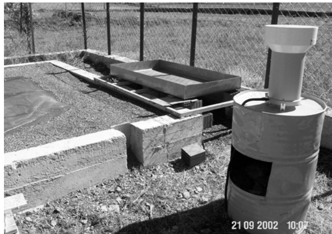
Figure 6: Tipping Bucket Rain Gauge.
