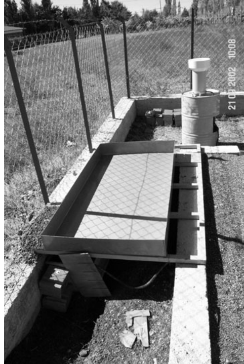
Figure 4: Snowmelt Lysimeter at Guzelyayla Station.
