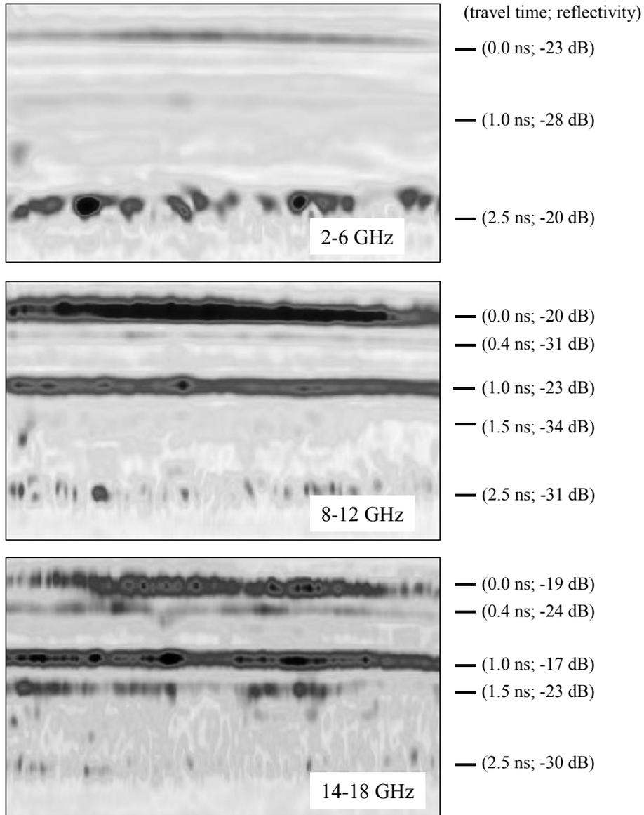
Figure 2. Multiband radar profile of a dry snowpack.
