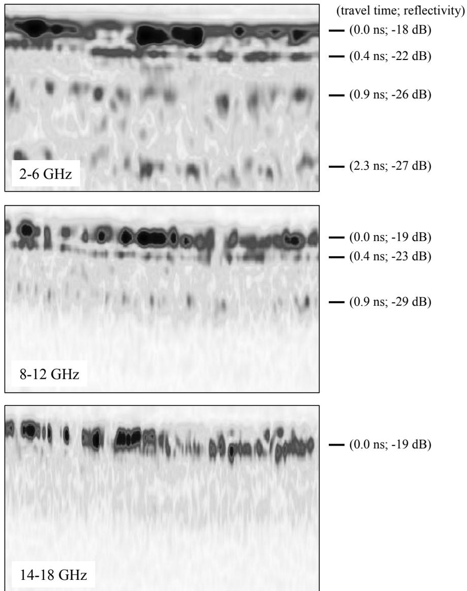
Figure 3. Multiband radar profile of a wet snowpack.
