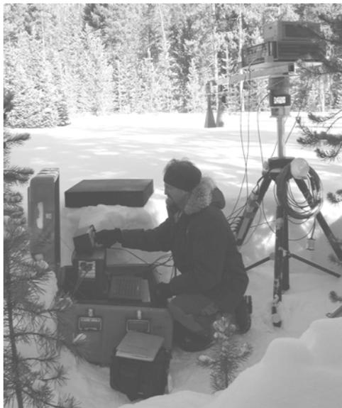
Figure 1. Ground-based FMCW radar.
