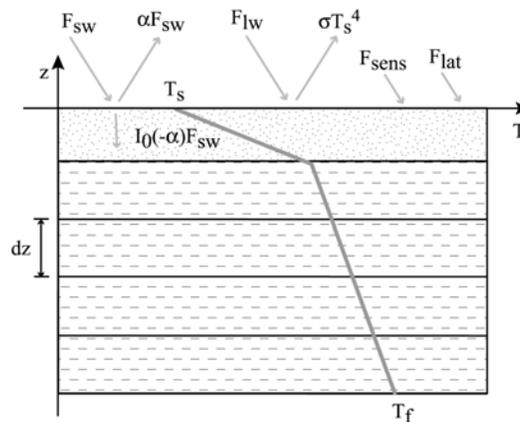
Figure 1. Schematic illustration of CLIMo under winter conditions.
