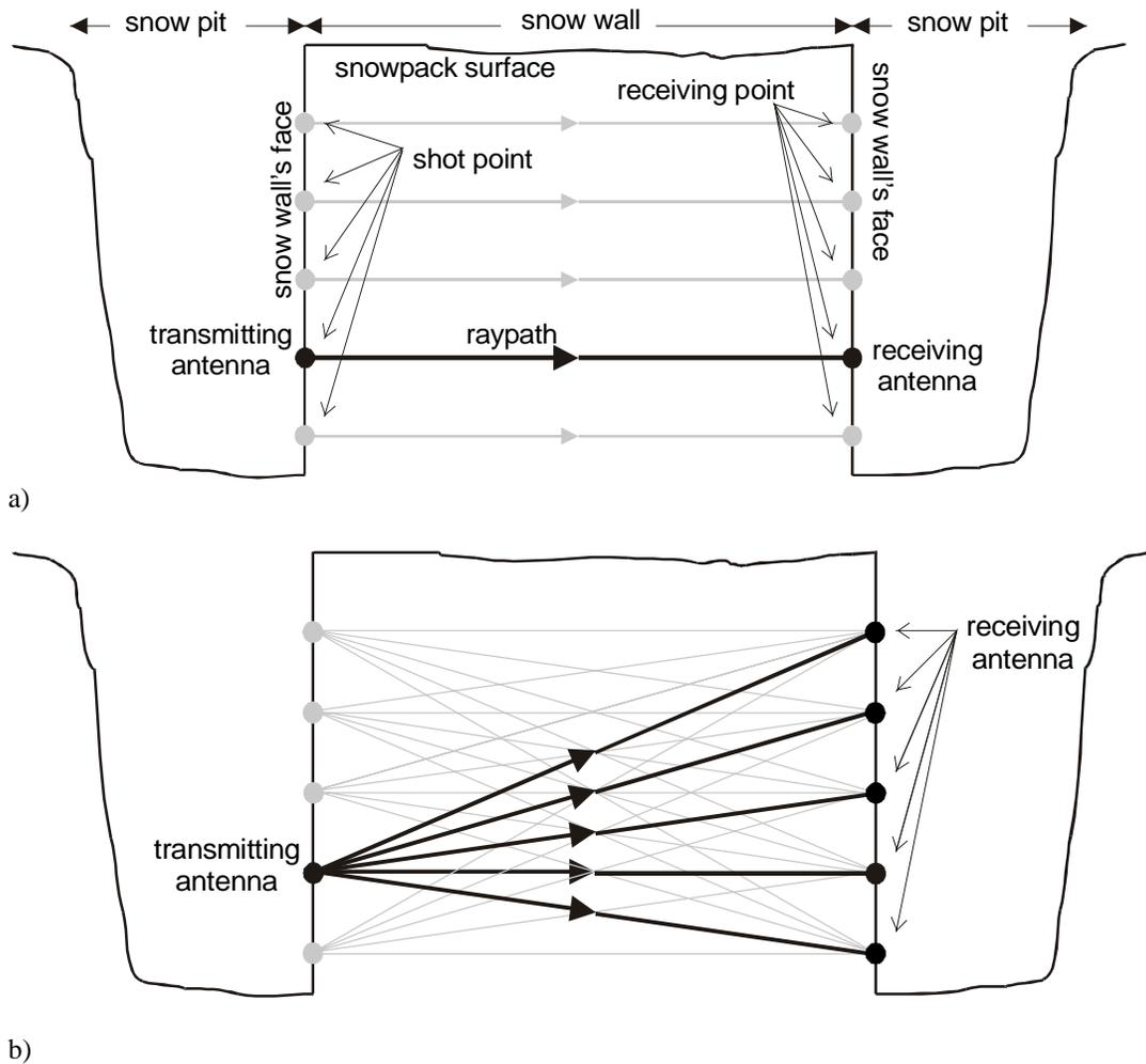
**Figure 2. A snow wall excavated in the snow cover where GPR pulse transmission can be performed. The GPR antenna are located along opposite side of the snow wall so that the EM pulse travel through the wall before reaching the receiving antenna.**
