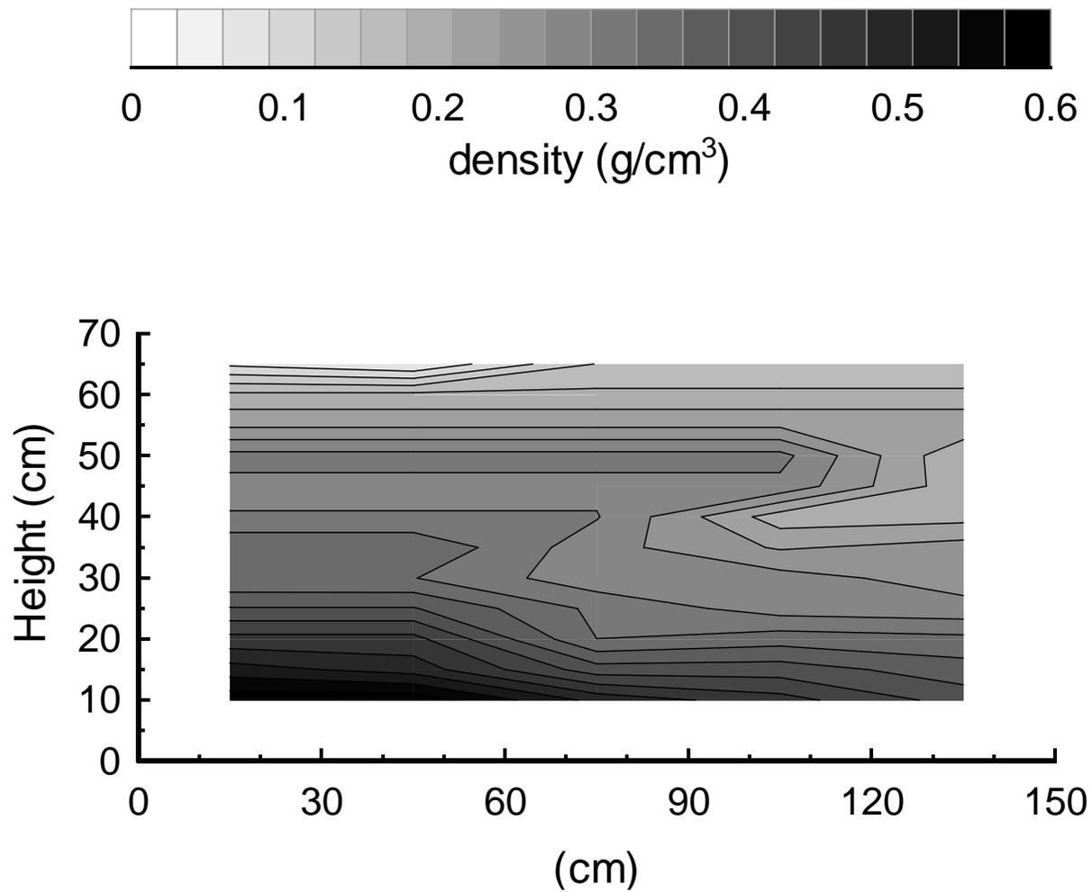
Figure 6. Tomographic image of the snowpack obtained with a bias-ART algorithm.
