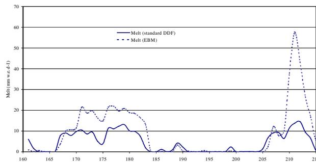
Figure 6. Melt calculated using EBM versus degree-day method.
